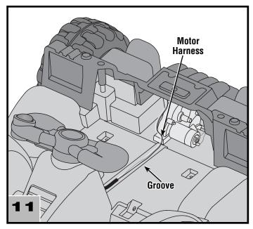
Fit the motor harness into the groove in the vehicle floorboard, as shown.
